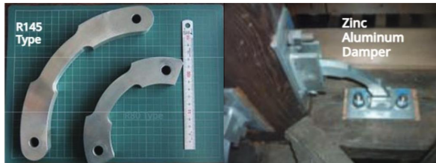
Figure 18. Zinc-Aluminum dampers (MOCHIZUKI et al., 2017) [35]
